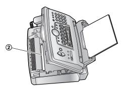
**12** Close the front cover (①) by pushing down on both sides, until locked.
